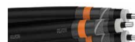
POLYCAB TRIPLEX ANTI-TERMITE MV AS/NZS 1429.1 6.35/11 (12) KV (Aluminium)
