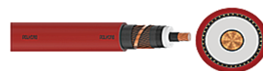
POLYCAB MV AL BS 7870-4-10 6.35/11 KV Triplex - Medium Voltage Copper wire screened Cable, 6.35/11 (12) KV AC
